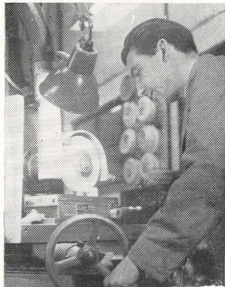
Mr. Frank Howells of the Grinding Department is working on the precise final finish of one of our special purpose tools.
